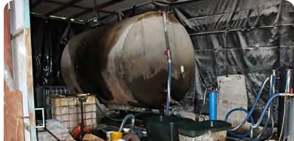
Fuel Laundering Plant where rebated diesel fuel is laundered/washed through 'cat litter' or 'fullers earth clay' material to remove colour from product.
