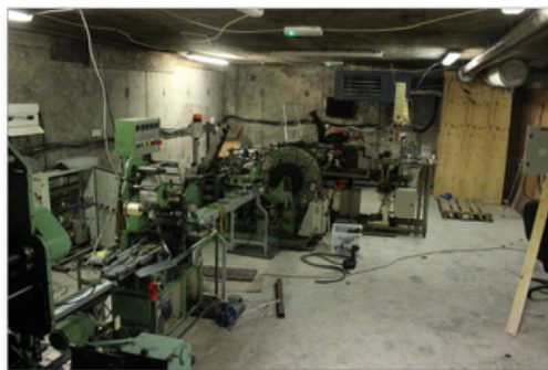
Industrial scale cigarette manufacturing machinery, in later stages of construction.
